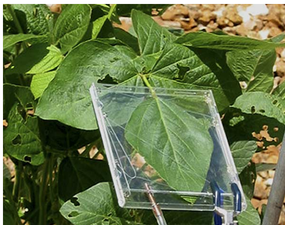
Fig. 2. The ^{13}\text{CO}_2 labeling of a soybean leaf using a compact-disc case as a labeling chamber. The labeling gas (21% \text{O}_2 , either 200 or 300-ppm ^{13}\text{CO}_2 , and the balance \text{N}_2 ) entered at the bottom left through a copper pipe closed at the end and with multiple exit holes along the sides. At the end of the labeling period, the leaf was cut from its stem, immersed in liquid nitrogen, and subsequently lyophilized.
